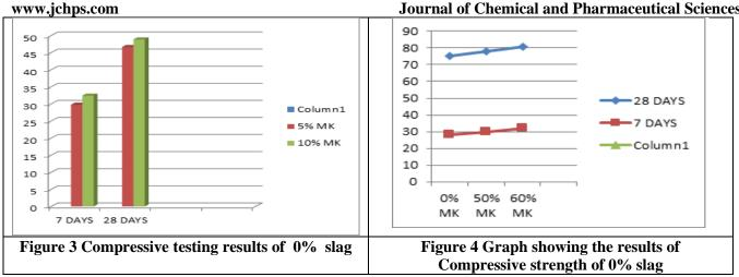
The value above indicates that there is an increase in compressive strength of concrete to a range of 6.5 to 13.4% is observed and is maximum at a replacement of 10% MK.
