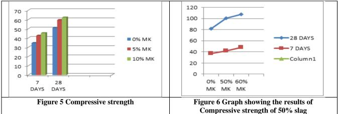
From the above results it is observed that by keeping the slag constant and by increasing the replacement of MK, the compressive strength is proportionately increasing with the increase of MK and by increasing the percentage of Metakaolin replacement are tested and shown below.
