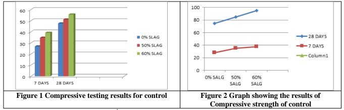
**Observation:** Here on seeing the 28<sup>th</sup> day results we find there is an appreciable increase of around 5% to 10% in the compressive strength when slag is replaced by cement and it also to be noted that the increase is more when the replacement is about 50%.
